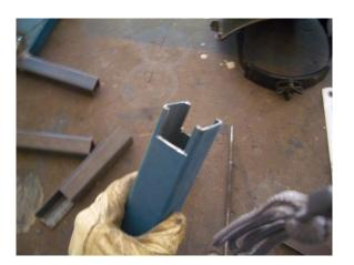
8. Position the cross bar and in the middle and weld in place
