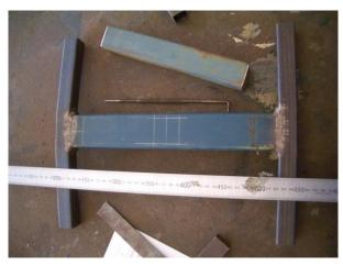
4. Once all marking out is complete position the vertical bars then tack weld in place and check for square. Tap the bars with a hammer to square up then finish weld in place.
