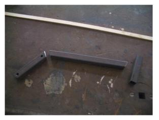
16. Tack weld all components in place then do a practice assembly to ensure that the jack works correctly and all components function as they should
