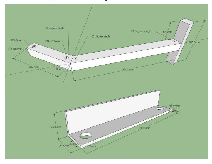
15. Cut all stock to length, mark and drill holes to 10mm.
