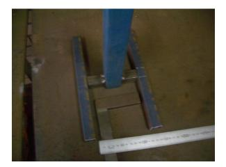
11. Weld in place and grid if required
