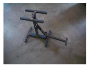
17. If required make the appropriate adjustments and re-test the function, then finish weld all parts of the jack and grind the required joints. Bolt together and test.
